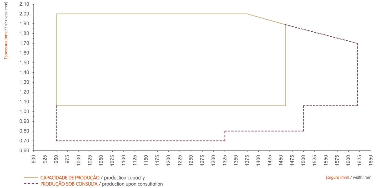
**BOBINA GALVANIZADA (GI/GL) - QUALIDADES INTERNAS AM01 E AM HSLA240**
