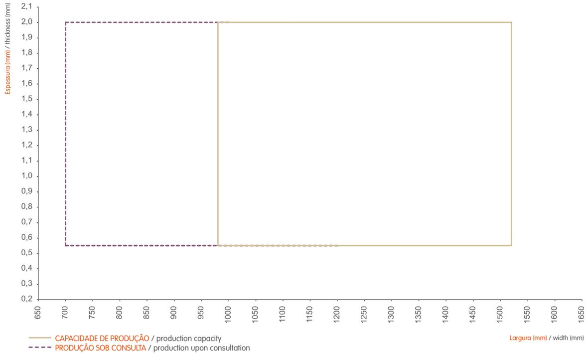
**BOBINA GALVANIZADA (GI/GL) - QUALIDADES INTERNAS AM HSLA 280, AM HSLA 320 E AM HSLA 360 - GALVANIZAÇÃO 2**
