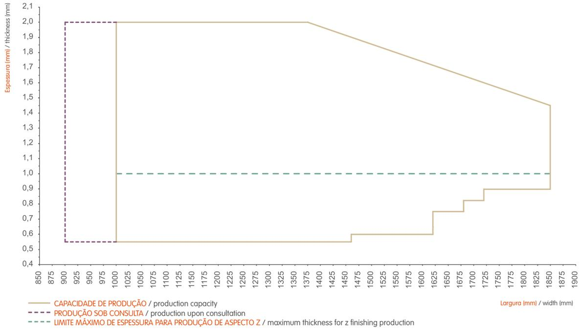
**BOBINA GALVANIZADA (GI/GA) - QUALIDADES INTERNAS AM H260PD E AM H280PD - GALVANIZAÇÃO 1**
